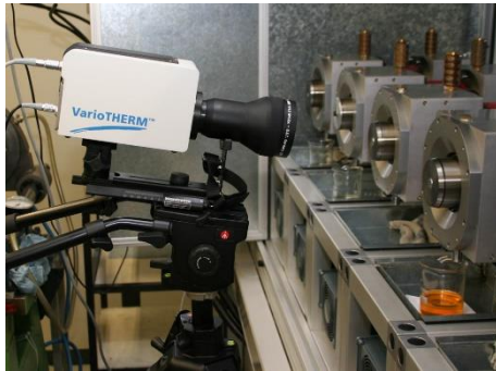
Infratec VarioTHERM II high-resolution thermographic camera on sealing ring endurance test bench
