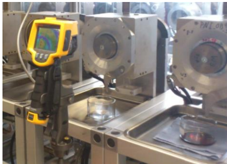
Hand-held Fluke Ti32 thermographic camera on sealing ring endurance test bench
