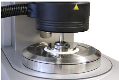
Cone plate Experimental set-up
