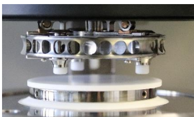
Tribology measuring system: "Pin-on-Disk" method
