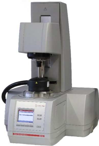
Rheometer "MCR 302" with temperature control cover
