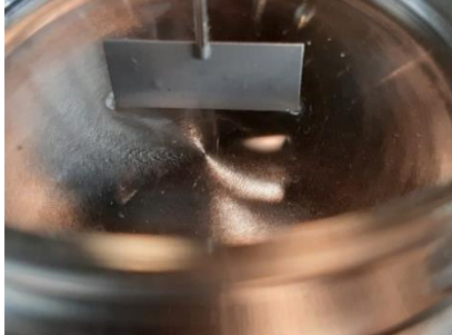
Measurement of the surface tension of lubricants by using the Wilhelmy-Tensiometry
