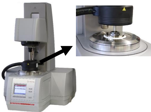
Rheometer with temperature control unit (left) and cone plate test setup (right)
